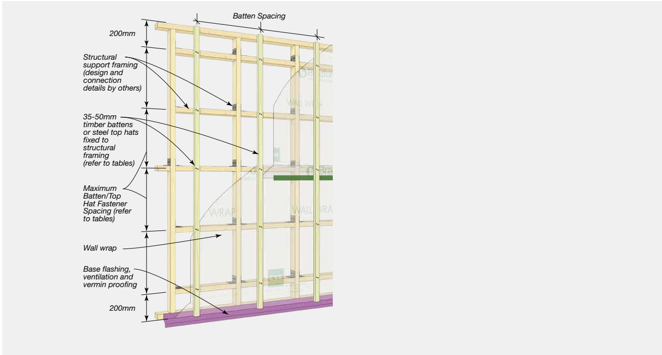
FIGURE 5.05 Typical Timber Batten Installation
