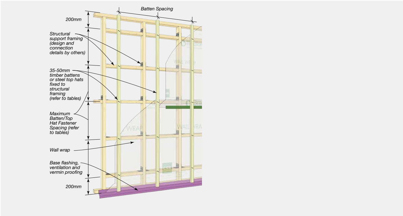
FIGURE 5.04 Typical Timber Batten Installation
