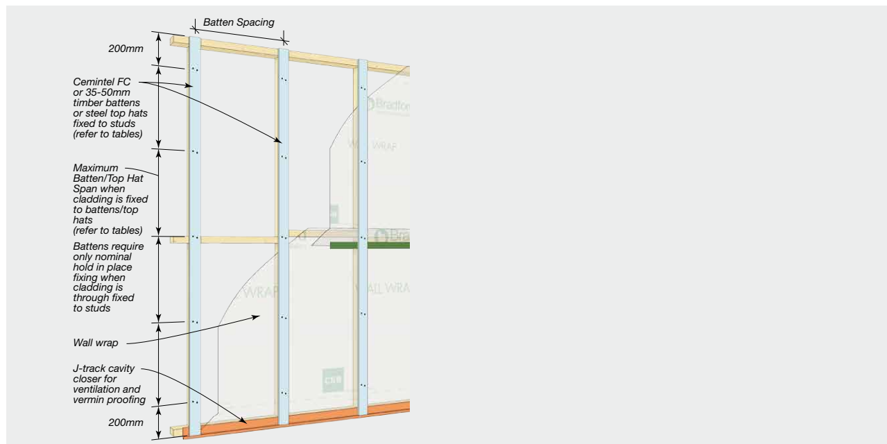
FIGURE 6.03 Typical Cemintel FC Batten Installation
