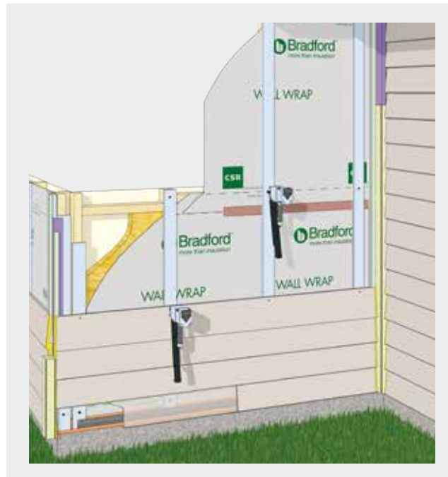
FIGURE 6.02 Cemintel Non-Structural Timber Batten Installation
