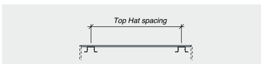
FIGURE 6.05 Panel Fixed to Two Top Hats Only
