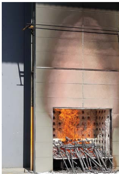
30mins - crib removed
