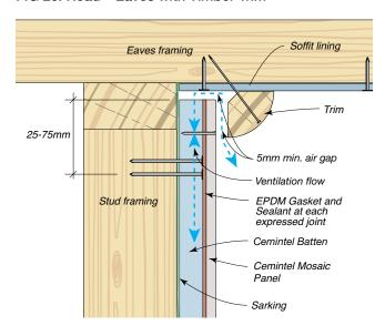
FIG 27: Soffit - With Cemintel Soffit Trim
