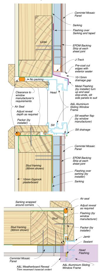
FIG 39: Dowell Sliding Door Installation – 70mm Framing and 85mm Reveal Shown
