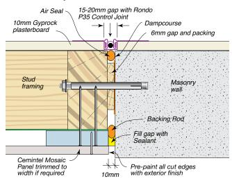
FIG 35: Junction of Mosaic Cladding System with Alternative Fibre Cement Cladding – Plan View
