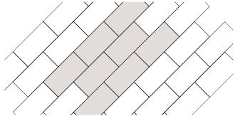
FIG 8: Diagonal Sheeting - Stack Bond Pattern
