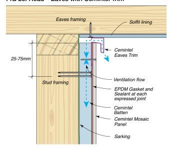
FIG 26: Head - Eaves with Timber Trim
