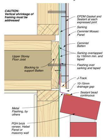
FIG 21: Second Storey Horizontal Junction
