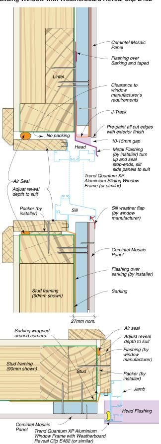
FIG 37: Window Detail – A&L Awning Window with Weatherboard Trim
