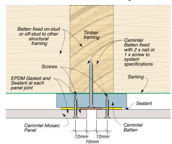
FIG 30: Horizontal joint
