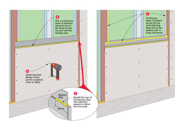
FIG 17: Base - Concrete Slab Foundation
