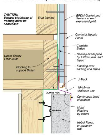
FIG 20: Second Storey Junction with Masonry, Brick Veneer or Hebel Panels In-line Framing
