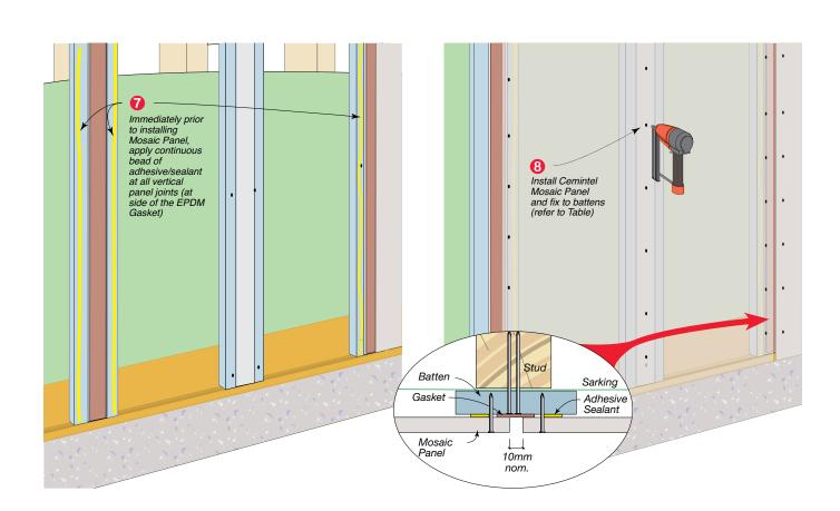
FIG 16: Installation Procedure - Vertical and Horizontal Joints
