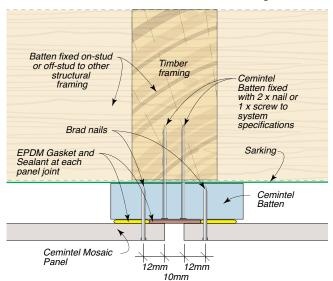
FIG 29: Vertical Panel Joint - Screw Fixing
