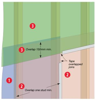
4 Horizontal flashings such as at the head of doors and windows, horizontal storey junctions and at the wall base (when used) require special treatment to ensure water is always shed towards the outside. Refer to appropriate junction details for specific requirements. A typical detail is shown below.
