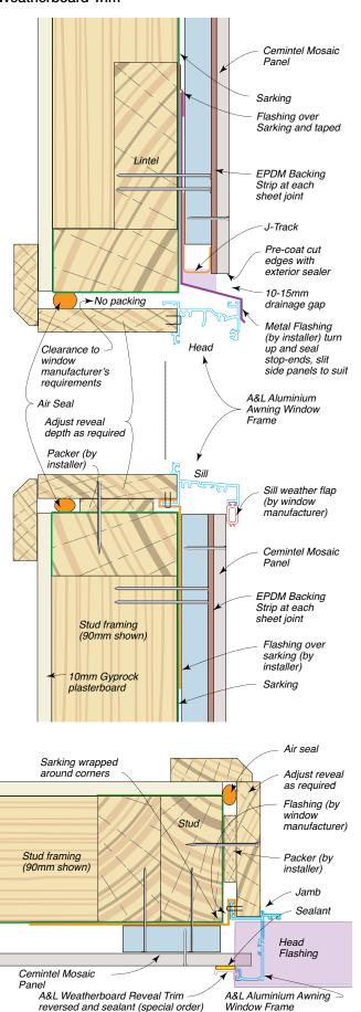
FIG 38: Window Detail – A&L Aluminium Sliding Window with Cladding Trim
