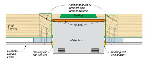
FIG 44: Power Meter Box Installation - Face Fix Installation
