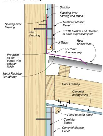
FIG 24: Horizontal Parapet Wall
