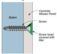
**HINT:** One way of applying filler is through a 20mm hole in thin metal sheet (0.6mm or less) or other suitable material. This will minimise spill-over and allow for some shrink back of the filler without having to repeat the application.
