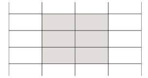
FIG 2: Horizontal Sheeting - Stretcher Bond Pattern
