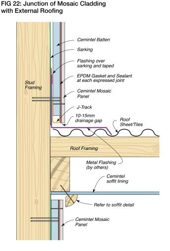
FIG 23: Junction of Mosaic Cladding with External Roofing
