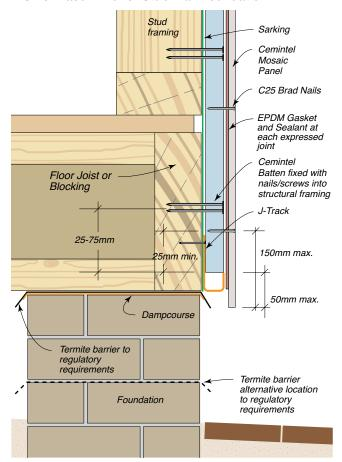
FIG 19: Second Storey Junction with Hebel Panels, Brick Veneer or Masonry Wall - Cantilevered Framing
