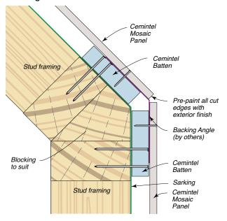
FIG 34: Junction of Mosaic Cladding System with Offset Masonry Wall – Plan View
