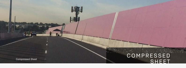
The strongest of them all, Cemintel Compressed Sheet is tried and tested for long term strength. Designed for use in tough conditions, including partitions and noise barriers, these panels have good acoustic properties and maximum impact resistance for a fibre cement product. The comprehensive range consists of multiple thicknesses, widths and lengths.
